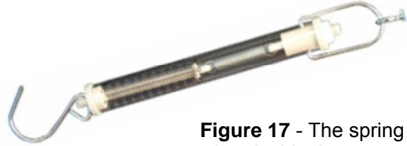
**Figure 17** - The spring when inside the calibrated casing [12]
