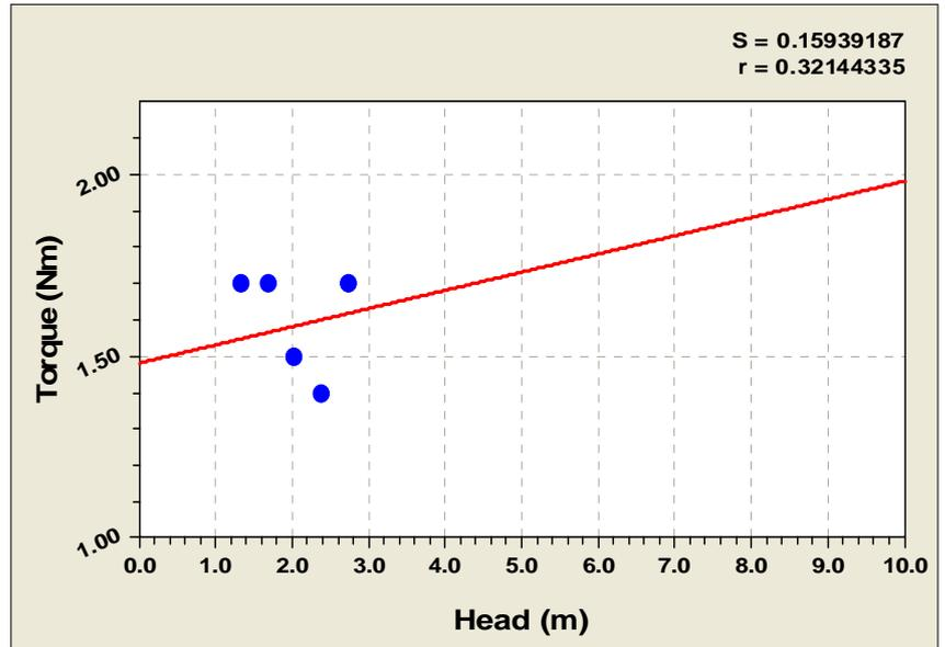
**Figure 26** - Line of best fit through measured torque against the height of head in the 19mm diameter pipe.
