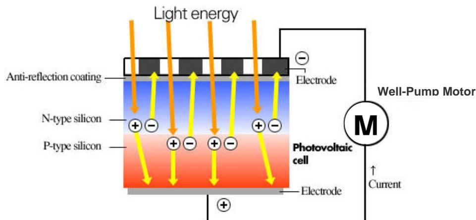
**Figure 4** - Illustration to demonstrate how a PV cell creates a current. <sup>[5]</sup>
