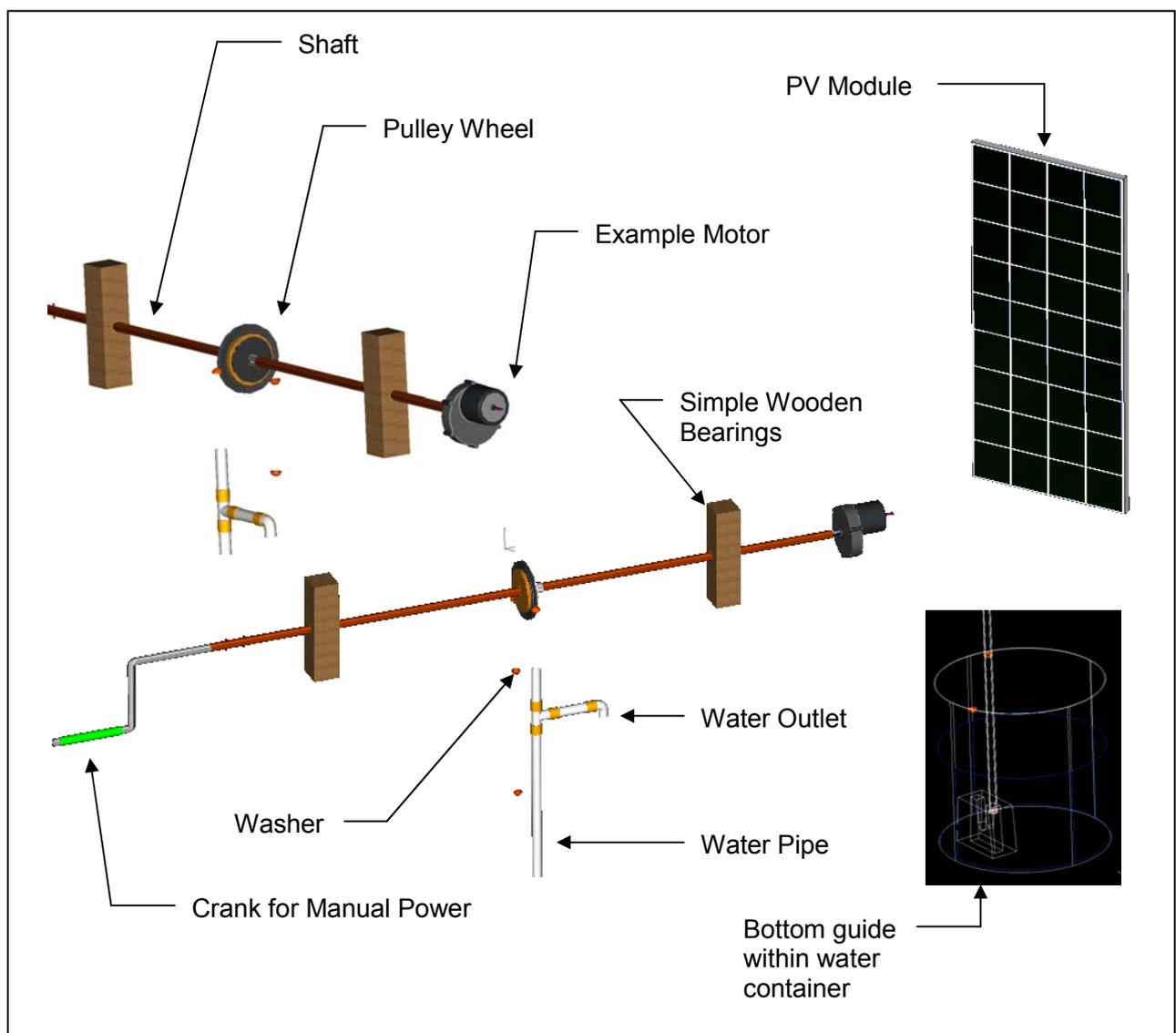
**Figure 11** – CAD models of fundamental parts of one third scale solar pump.
