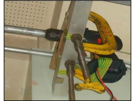
**Figure 16**– drill mounted to crossbeam for fuller shaft support
