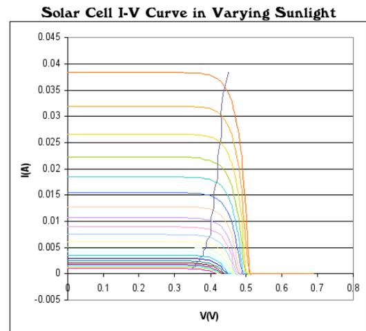
**Figure 10** - Thin blue line hits each knee to find max power <sup>[10]</sup>
