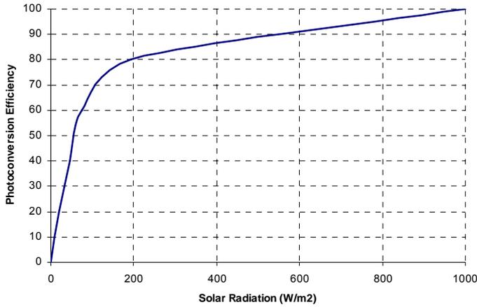
**Figure 5 - Efficiency against Solar Radiation**<sup>[6]</sup>
