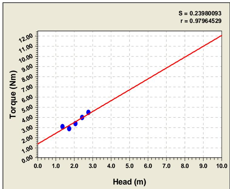
Figure 24– Graph to represent results, and line of best fit, of measured torque against the height of head in the 36mm diameter pipe.
