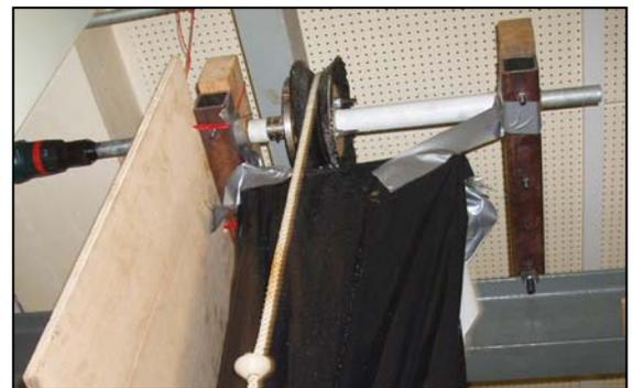
**Figure 13** - Shaft supported by series of brackets and girders.
