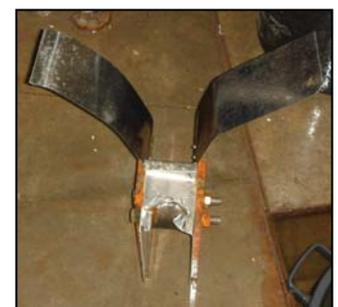
**Figure 14** – Heavy duty bottom bracket – experimental purposes only.
