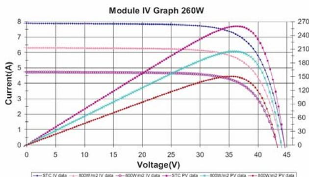
**Figure 28** – IV characteristics of a large 260W Solar Panel.
