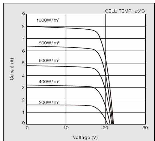
**Figure 8b - Current-Voltage characteristics of Photovoltaic Module KC130TM at various irradiance levels.**<sup>[8]</sup>
