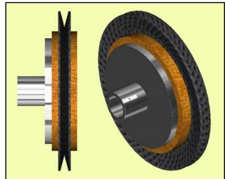
**Figure 15** - CAD model of second pulley wheel design
