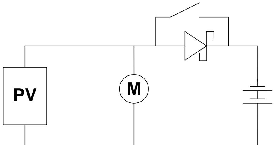
**Figure 29** – Solar Module Circuit including Battery
