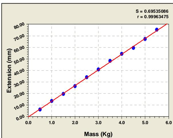
**Figure 21** (right) – Graph of spring extension against force applied. The correlation coefficient (r) is very high; indicating the equation for the line of best fit can be relied upon.
