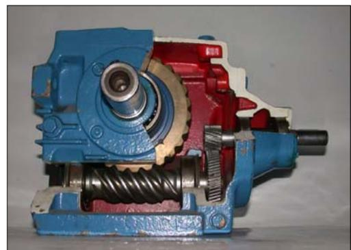
**Figure 25** – Cut-out section of Worm & Wheel Gearbox <sup>[14]</sup>
