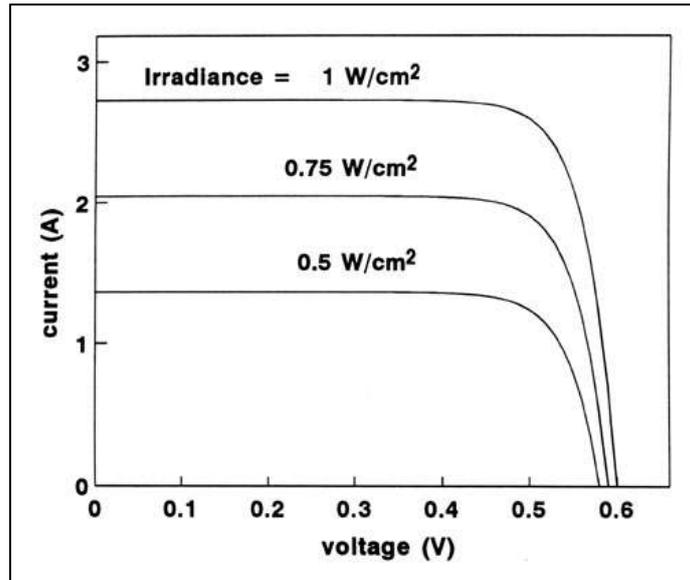
Figure 3: Effect of varying insolation on the I-V curve of a ~1.5W PV cell (adapted from [21])
